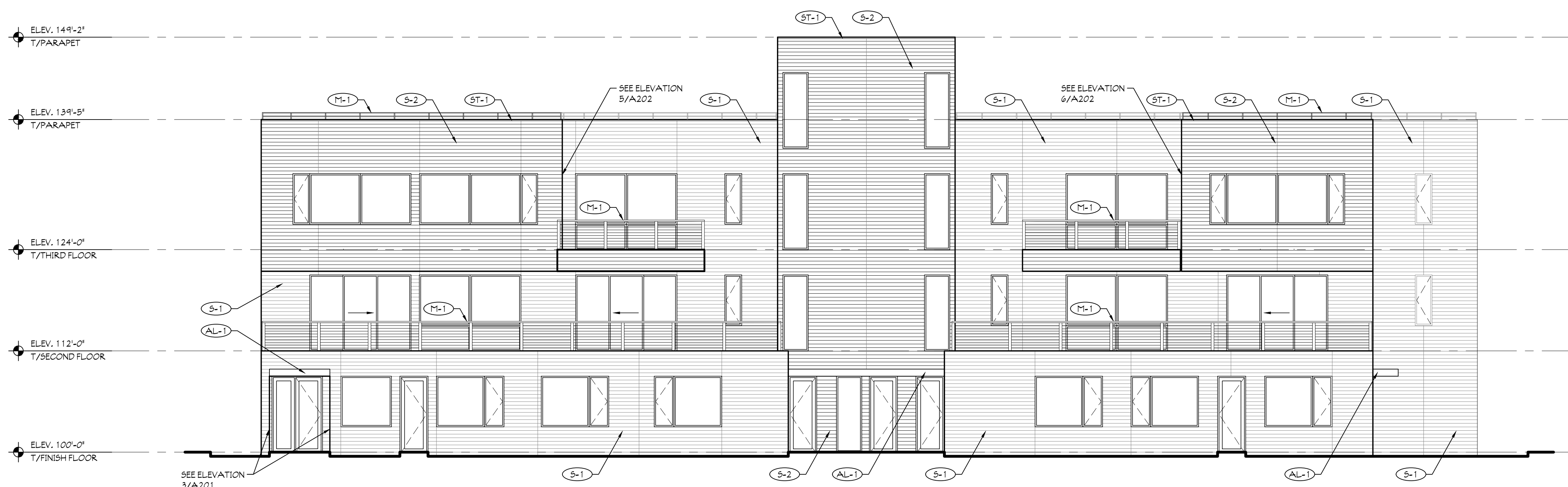
1 NORTH ELEVATION SCALE: 1/8" = 1'-0" BUILDING #2
