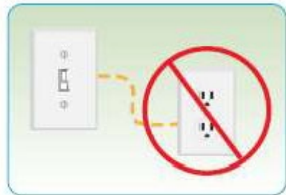
Do not use outlets that are controlled by wall switches.
